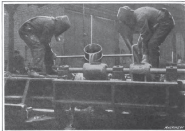
Fig. 6. Pouring Clamping Metal. Attention is called to Arrangement of Clay to hold Molten Metal in Place until it solidifies
